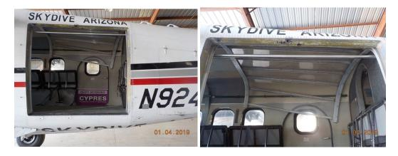
Door measurements are 127 cm. high and 140 cm. wide. A floater bar the length of the door is inside the plane. 84 cm. behind the door, on the same level as the floor, is a videographer's step. Above and behind the door are videographer handles.
